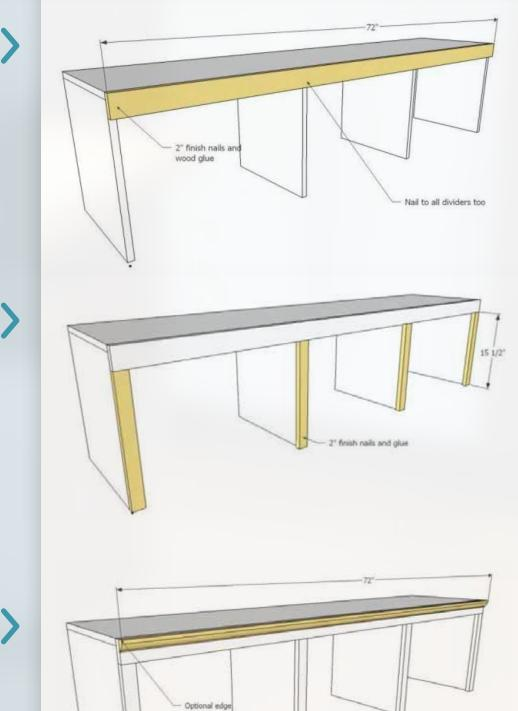
moulding attached with 1 1/4" finish nails and wood glue
