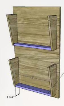
Attach to sides and base using glue and 1-1/4" brad nails.
