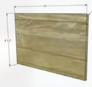
Cut a 12 deg. bevel in both the top and bottom.
